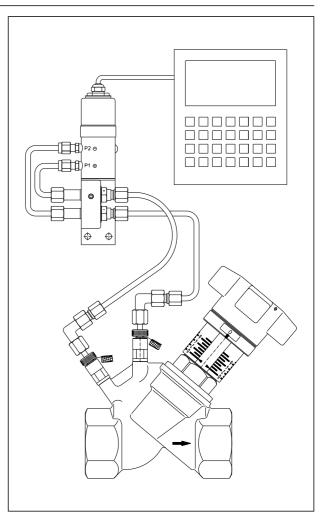
Example of installation differential pressure transmitter
