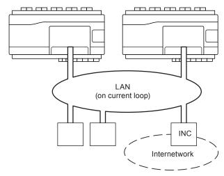
Note: In this configuration the IQ3 cannot join a Trend LAN on Ethernet. However, access by IP is still possible.
