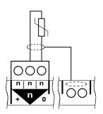
Voltage input: Used with a 0 to 10 Vdc source.
