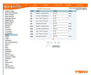
The web interface does not allow the strategy structure to be modified (e.g. changing module interconnections, adding or deleting modules). Graphical display pages (GraphIQs), which are configured using IQ3's Display and Directory modules, can also be accessed.
