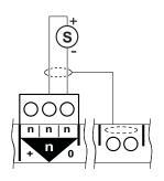
**Digital input:** Used for a volt free contact, logic circuit (e.g. TTL, CMOS), open collector (transistor) or open drain (FET).
