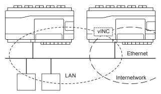
In addition, the IQ3 has the ability to join an internetwork using its virtual INC (see "Networking" on page 3 for further details).
