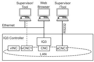
**sCNC1 Functionality:** If the RS232 port address is set to 0 (default), sCNC1 is disabled and a connected device can only communicate with the IQ3. If the address is configured to be non-zero, sCNC1 is enabled with that address on the LAN and allows a connected device to communicate with the entire Trend network.
