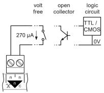
The volt free contact has a nominal wetting current of 270  $\mu A.$  The input is ON when the contact is closed.
