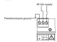
Note: Connection to the IQ4E is polarity independent.
