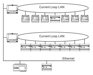
The diagram above shows IQ41x/LAN replacing/extending an IQ21x system on the Trend current loop LANs, and an IQ41x connected to a Trend Ethernet LAN.
