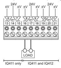
**IQ41x/230:** Switches 24 Vac (synthesised), 300 mA maximum for a channel, 300 mA maximum shared between all (4 or 6) channels. Terminals and example wiring:
