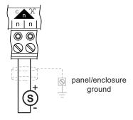
**Digital input:** Used for a volt free contact, logic circuit (e.g. TTL, CMOS), open collector (transistor) or open drain (FET).
