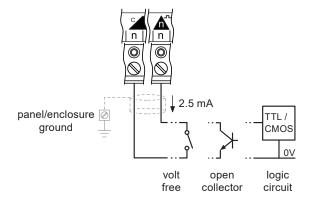
The volt free contact has a nominal wetting current of  $2.5\,$  mA. The input is ON when the contact is closed. There is no polarity.
