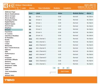
The web interface does not allow the strategy structure to be modified (e.g. changing module interconnections, adding or deleting modules).
