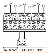
Each output provides an independent 24 Vac feed for driving 24 Vac loads, such as thermoelectric (thermic) actuators, and raise lower actuators, (e.g. the Trend range of thermic actuators).
