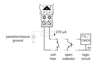
The volt free contact has a nominal wetting current of 270  $\mu\text{A}.$  The input is ON when the contact is closed.
