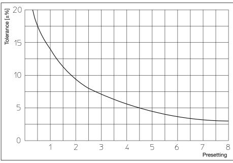
Flow tolerances depending on the presetting for DN 65 – DN 150
