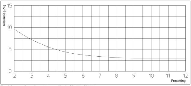
Flow tolerances depending on the presetting for DN 200 – DN 300
