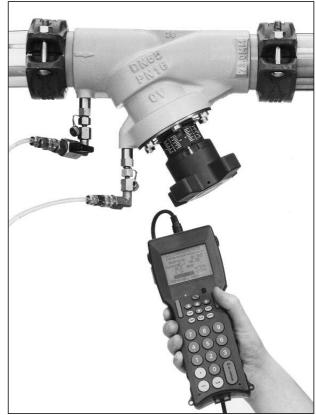
Flow meter "OV-DMC 2", item no. 1069177 with "Hydrocontrol VGC" DN 65
