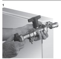
After having removed the thermostat from the valve, slightly loosen the valve insert with the help of a corresponding tool (M 30 x 1.5 spanner size 19 / M 30 x 1.0 spanner size 17). The "Demo-Bloc" is now screwed onto the valve.
